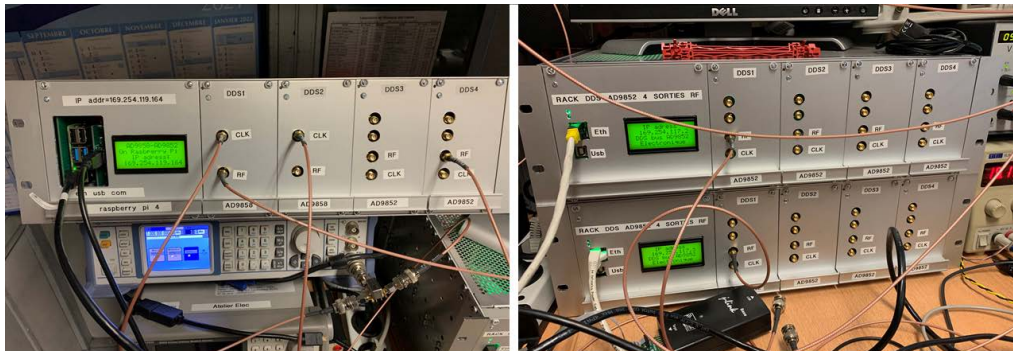
DDS boards for Laser Superradiant experience (Strontium 2)
